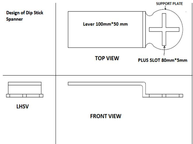
Fig 3: 2d Design of Dip Stick Spanner.
