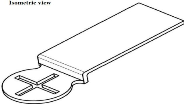
Fig 2: 3d Design of Dip Stick Spanner.
